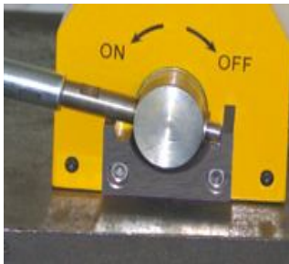
1. Handle locked in Demag (OFF) position
