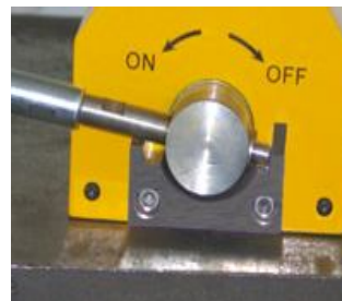
5. Handle locked in Mag (ON) position
